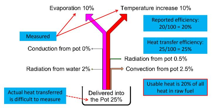
During a heating cycle, the losses from the pot are provided and the net heat gained by the water can be determined observing the change in temperature and evaporated water mass. The measured heat transfer efficiency is lower than the actual efficiency as not all heat losses can be measured. Heat getting into the pot is 25% of the heat in the fuel, but only 20% is useful.
