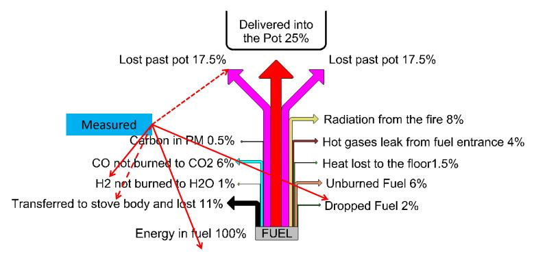
Some fuel energy paths can be measured easily (solid red lines). Heat flow is easier to evaluate than heat in unburned fuel. Losses are chemical, mechanical or wasted heat in gases. "Heat Transfer Efficiency" to the pot is 25% of the heat available in the raw fuel.
