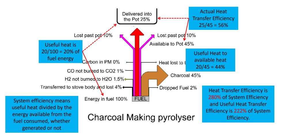
Heat Flow Diagramme for the charcoal maker — Thermal efficiency determined using a boiling or cold pot, high or low power, produces very different results for the same metric
